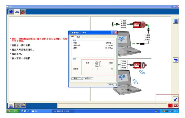
8, to make sure VCM and PC have a good communication, open Local Links, to see its data package, the "receive" and "send" must be balance, if it is not balance, to make sure close "firewall".
