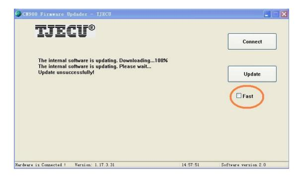
Step 5: After remove the Hook in front of Fast then press Update button. After then CN900 and update with computer together.
