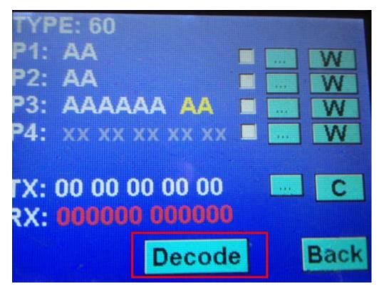
After click the Decode button then it start to decode. (Notice: Do not move the 4D key which you want to copy)
