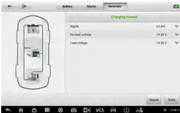
Figure 9-12 Generator Test Result Screen
