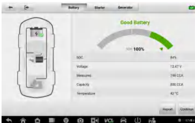
Figure 9-7 Battery Test Result Screen
