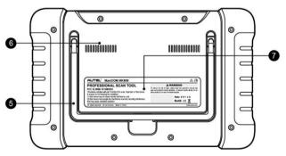
Figure 2-2 MaxiCOM MK808 Display Tablet Back View
