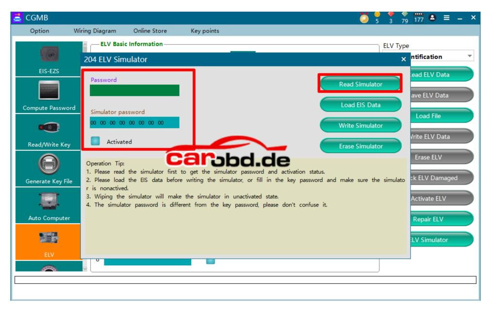
The fourth step is to read the simulator to ensure that the simulator is inactive. If it is activated, please wipe it first.
