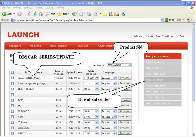
5) One-by-one to download DBSCAR\_SERIES-UPDATE, firmware upgrade package, X431 IV DISPLAY and car models software.
