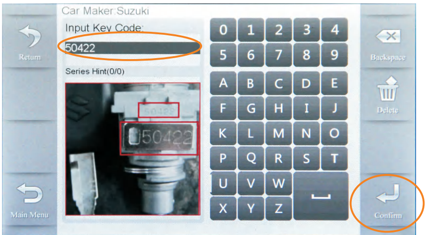
3) Enter the key code (the key code is printed on the lock for some cars) and click 'Confirm'.
