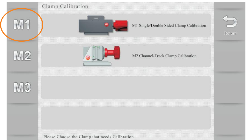
3) Select clamp M1 and proceed by following the tips on the screen.
